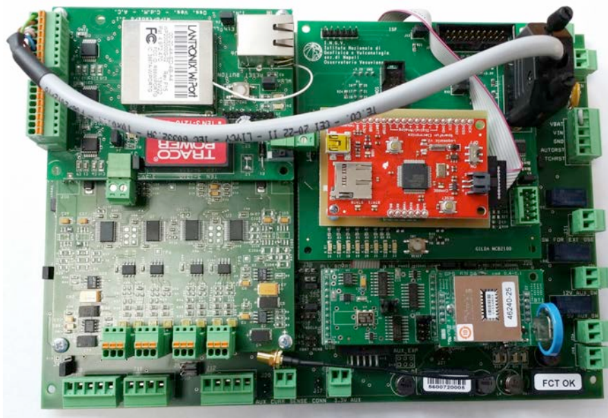
Figure 1. An example of a GILDA system: it is possible to detect the WiFi module, the main ADC and, in red, the board to write data to an uSD card.
