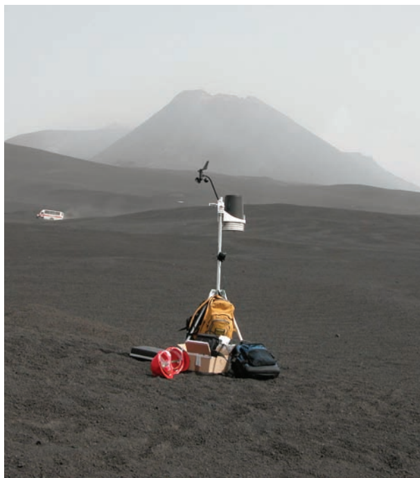
Figure 5.15 Davis Vantage Pro meteorological station.
