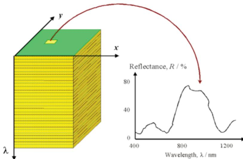
**Figure 1** An illustration of a hyperspectral image cube. The hyperspectral image data usually consists of over a hundred contiguous spectral bands, forming a three-dimensional (two spatial dimensions and one spectral dimension) image cube. Each pixel is associated with a complete spectrum of the selected area.
