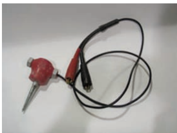
Figura 33 Sismometro Mark L-15B a componente verticale (www.ce.unlv.edu/egL/Equipment). Figure 33 Vertical component Mark L-15B seismometer (www.ce.unlv.edu/egL/Equipment).
