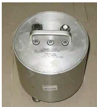
Figura 34 Sismometro a tre componenti Mark L4-3D (www.ija.csic.es). Figure 34 Three-component Mark L4-3D seismometer (www.ija.csic.es).
