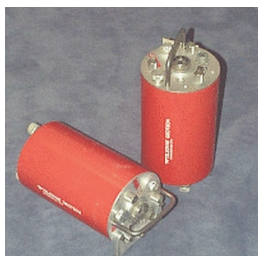
Figura 36 Sismometro Geotech S-13 a componente verticale ed orizzontale (www.geoinstr.com). Figure 36 Vertical and horizontal component Geotech S-13 seismometer (www.geoinstr.com).
