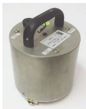
Figura 39 Sismometro a larga banda Guralp CMG-40T (www.guralp.com). Figure 39 Broad band Guralp CMG-40T seismometer (www.guralp.com).
