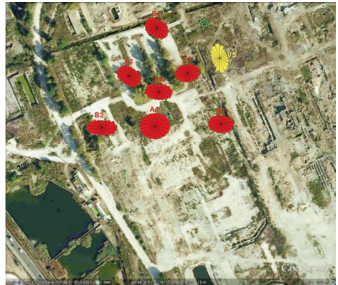
Figure 10 Rose diagrams of the polarization azimuth in the 1-5 Hz frequency band for data recorded during the November survey. The bins of the rose plots were chosen equal to 20°, to account for the uncertainties in the azimuth values. The data of the short period sensor VS are represented in yellow. The green star corresponds to the location of the drill.
