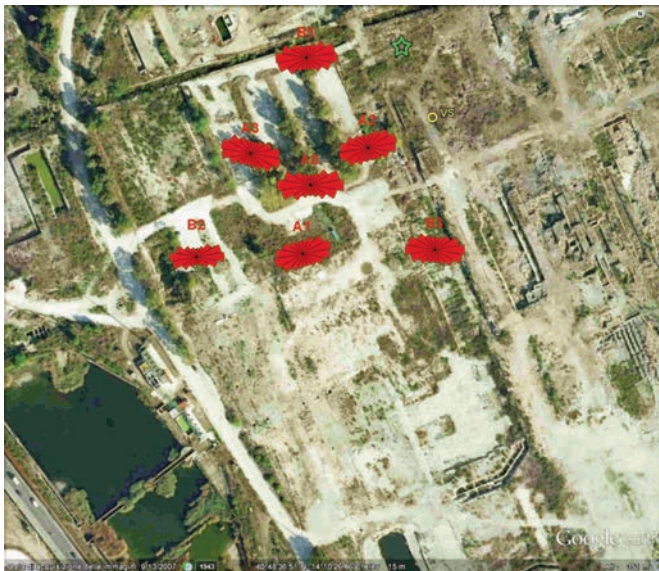
Figure 8 Rose diagrams of the polarization azimuth in the 0.1-1 Hz frequency band for data recorded during the November survey. The bins of the rose plots were chosen equal to 20°, to account for the uncertainties in the azimuth values. The data of the short period sensor VS are not reported for this frequency band. The green star corresponds to the location of the drill.
