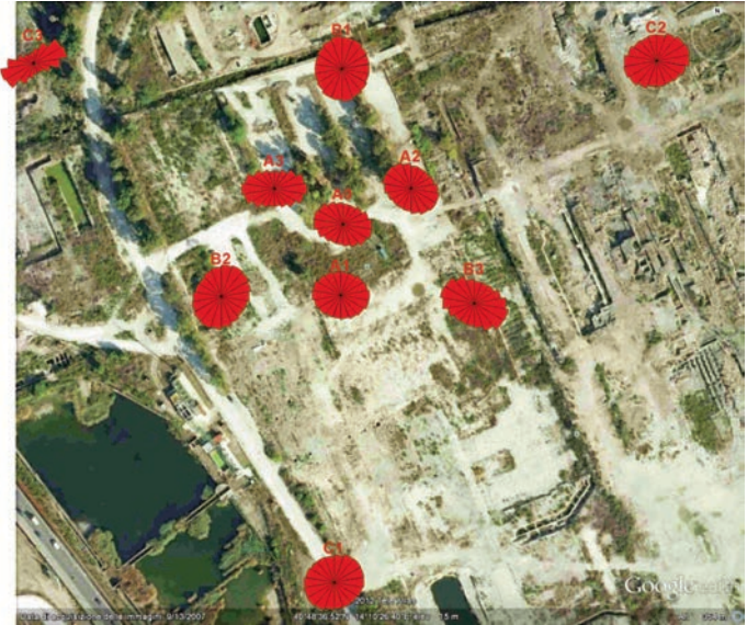
Figure 9 Rose diagrams of the polarization azimuth in the 1-5 Hz frequency band for data recorded during the April survey. The bins of the rose plots were chosen equal to 20°, to account for the uncertainties in the azimuth values.
