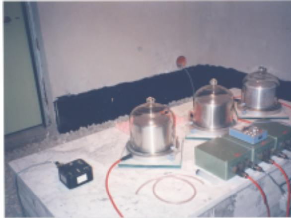
Fig. 6 – Basement of instrumentation: on the left the accelerometer FBA-23, on the right the three sensors STS-1.
