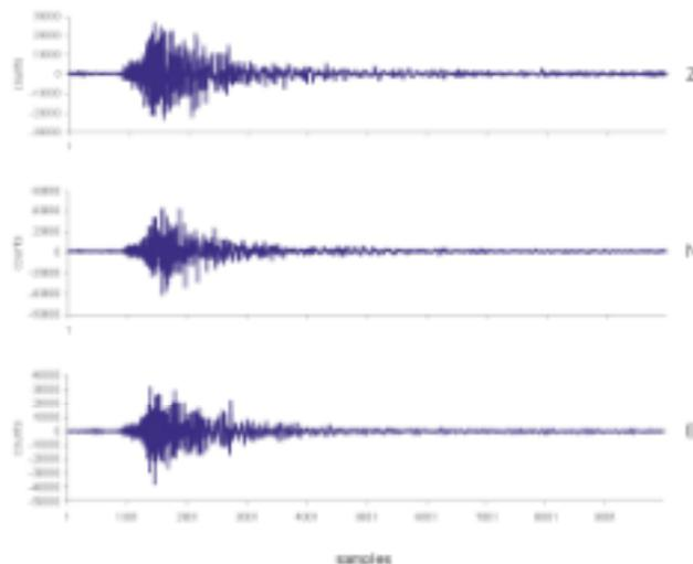
Fig. 9 – Example of a seismic event recorded by Q680 with a 20 Hz sample rate. From top to bottom: vertical (Z), north-south (N) and east-west (E) components.
