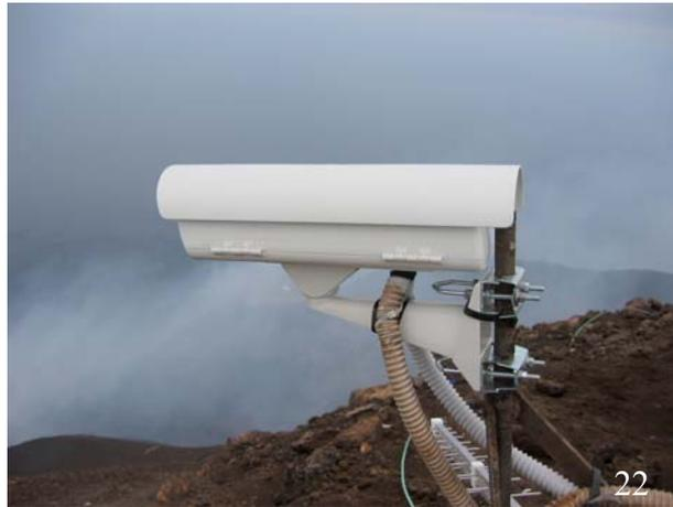
**Figura 22.** Telecamera Intellisystem ITTCC5 installata a “Il Pizzo Sopra la Fossa”.
