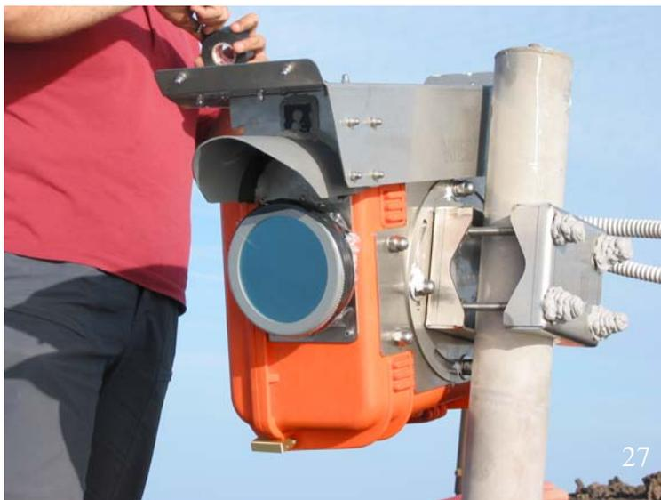
**Figura 27.** Telecamera Opgal. EYE – M 320B installata a “Il Pizzo Sopra la Fossa”.
