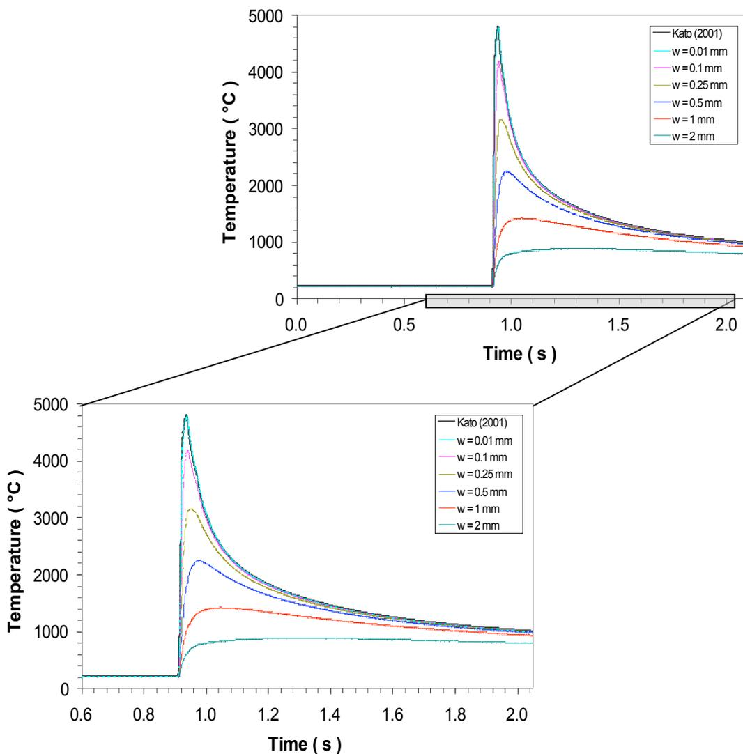
**Figure 4.** Effects of the different values of the thickness of the slipping zone (values are reported in the legends). Thick, black curves reports the solution by Kato (2001) for a better comparison. Bottom panel display a zoom in the time window marked on the top panel.
