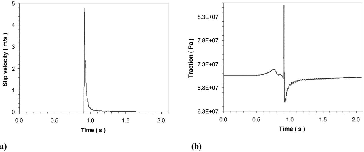
**Figure 2.** Time evolutions of the fault slip velocity (panel (a)) and traction (panel (b)) considered for the comparison between the two solutions for the temperature field. The solutions pertain to a fault receiver located at hypocentral depth and sufficiently far from the hypocenter and from the fault boundaries.
