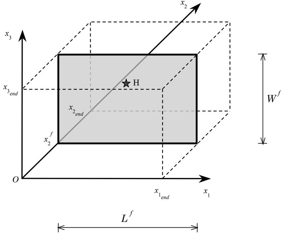
**Figure 1.** Schematic representation of the fault model considered in the present study. The grey plane  $x_2 = x_2^f$  represents the fault, the star H indicates the hypocenter. Dashed lines denote the spatial extension of computational domain,  $\Omega^{(FD)}$ , having dimension  $x_{1\_end}$ ,  $x_{2\_end}$  and  $x_{3\_end}$  in each direction. The plane  $x_3 = 0$  is the free surface.
