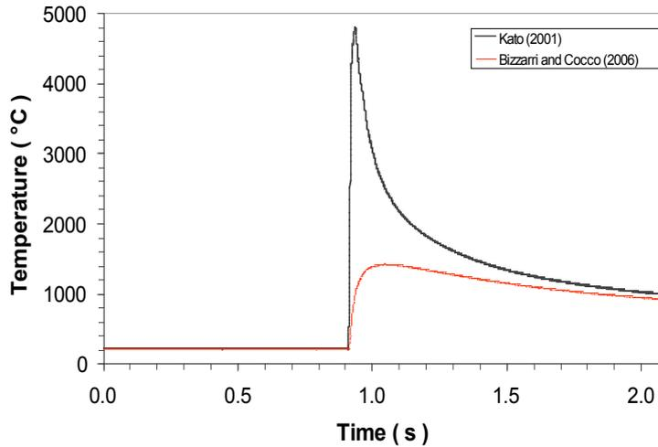
**Figure 3.** Comparison between the two solutions for the temperature evolution for the time histories reported in Figure 2.
