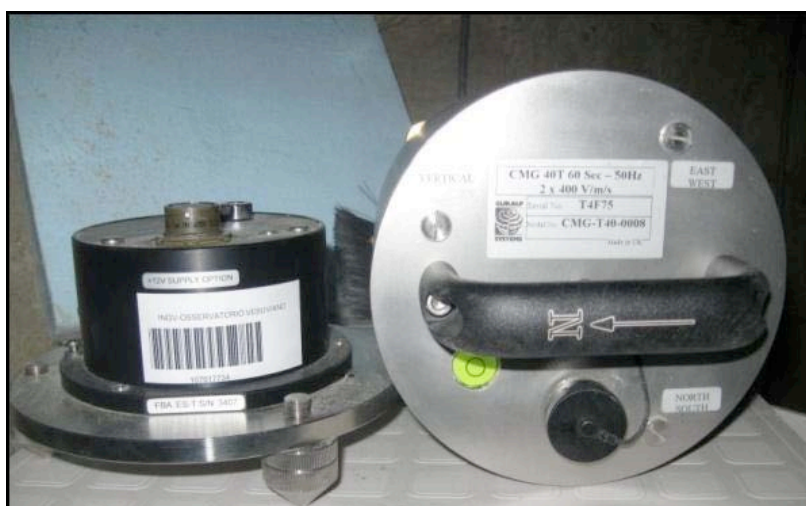
Figura 6. Accelerometro EpiSensor Es-T, a sinistra; velocimetro Guralp CMG40-T a destra.
