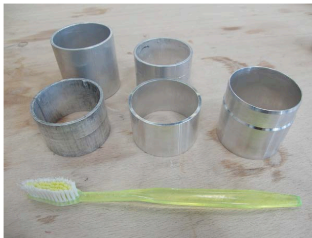
Figure 1. Metal rings: (left) original tube cuts, one used, one new; (middle) rings with rectified outer diameter for dry experiments; (right) rings rectified with profiling for use with pressure vessel. Toothbrush for your personal hygiene.
