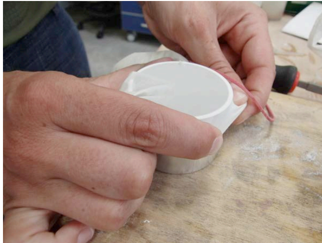
Figure 4. Seal bottom of ring with latex.
