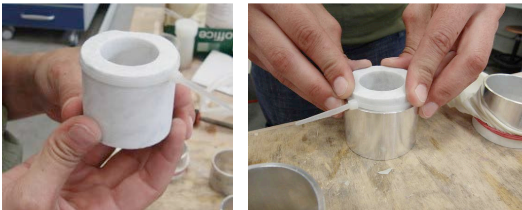
Figure 3. A nylon cable tie is wrapped close to the top of the sample. The rock sample is pushed into the ring until the desired height remains exposed at the top. The uglier, irregular side of the sample faces toward bottom. The nylon tie may be used in order to position the height. Note that the final adjustment of the exposed height will be rectified later using the lathe, so leave a little more than the final height.
