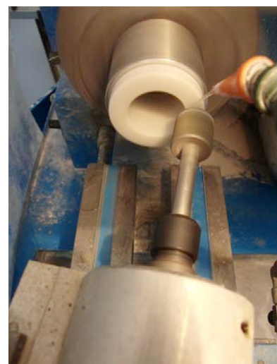
Figure 10. Approximate drill cylindrical bit to the sample top, the drill axis should make an angle of a few degrees with the late rotation axis (left). Turn on water and adjust the water gasket so that water is dripping on the sample. Spin direction: there are several possibilities depending on whether you set the drill at the far or close end of the SAMOA, and whether you make the angle in one direction or the other. Just always think that at the contact point between rock and drill bit, the tangential motions should be opposite in order to maximize mutual speed.
