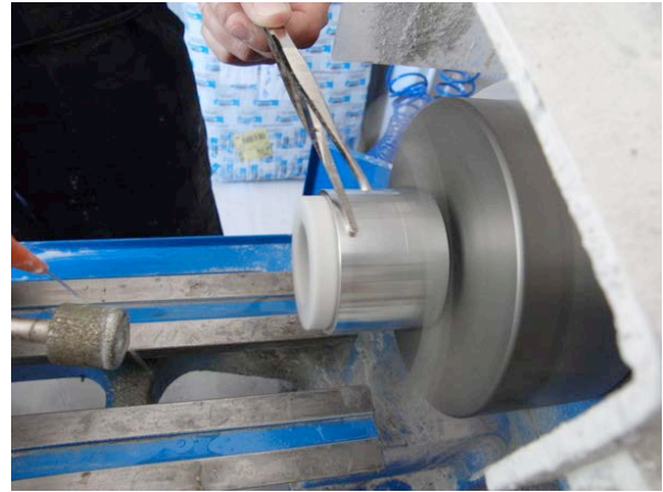
Figure 8. Fix the SAMOA in the lathe. BE CAREFUL! Make sure you removed all mobile parts (keys,...) from the mandrel before starting the machine. Do not put hands or objects too close to the claws. Check smoothness of rotation and centering: an object on the metal surface should not vibrate or jump (right).
