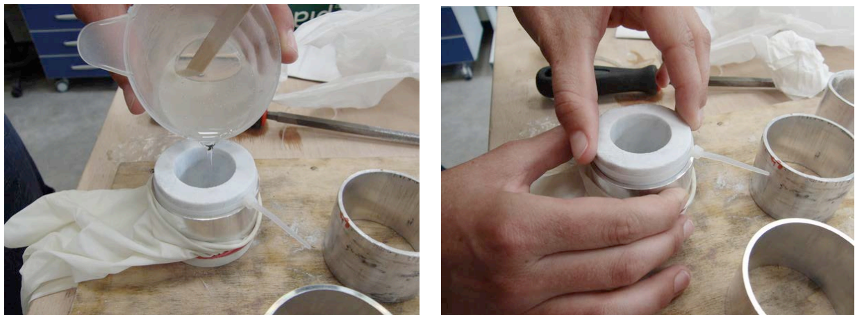
Figure 5. Sit sample, ring and latex on a flat surface. Mix epoxy resin. Pour in resin. Move sample up and down into ring to make sure that epoxy covers effectively the walls between rock and metal. Normally epoxy rises also by capillarity, if the spacing between ring and rock is tight.
