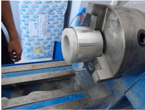
Figure 8. Fix the SAMOA in the lathe. BE CAREFUL! Make sure you removed all mobile parts (keys,...) from the mandrel before starting the machine. Do not put hands or objects too close to the claws. Check smoothness of rotation and centering: an object on the metal surface should not vibrate or jump (right).
