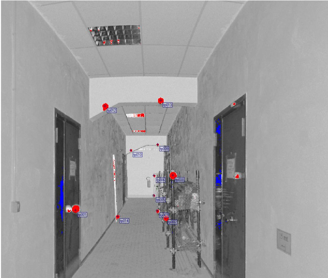
**Figure 7.** Scanning detail of overview with the identification of tiepoints.
