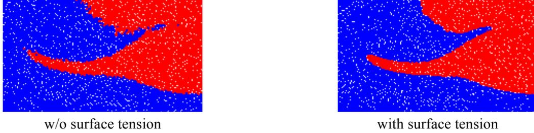
**Figure 5.** Evolution of the two-dimensional Rayleigh-Taylor problem, obtained with our implementation of Grenier’s method and using the simplified surface tension model with  $\varepsilon_l = 0.01$ . Particles are colored by fluid number.
